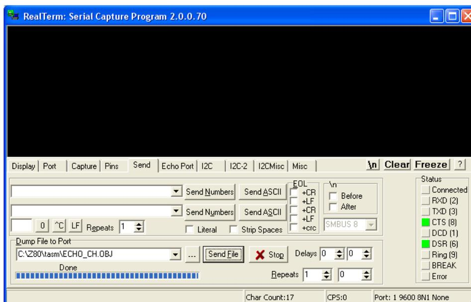
Now click the mouse in the RealTerm display window, and type on the keyboard. You should see your characters being echoed onto the display (and on the port 0 LEDs):
