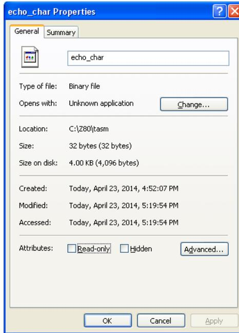
This file can be loaded back into the Z80 using blood. I first entered FFs into the Z80 memory at 0900h using the load command before loading back the file so you can see that it is really now just 32 bytes long:
