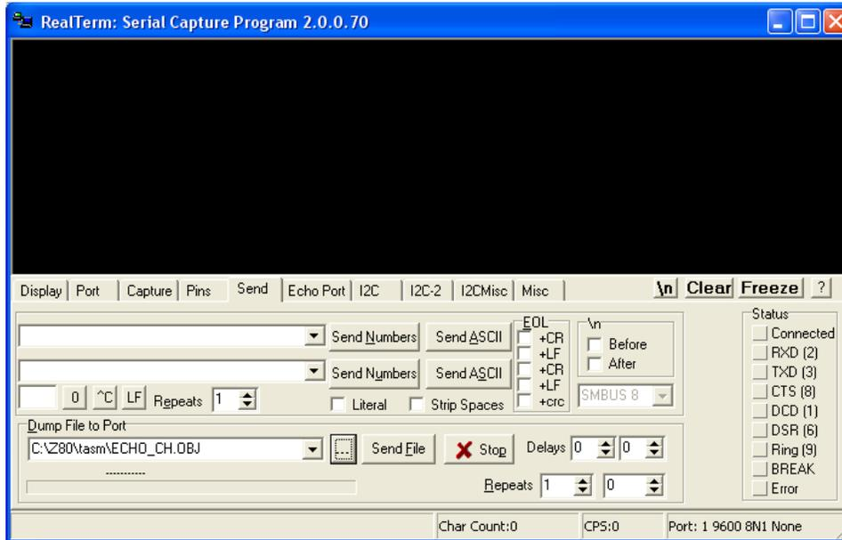
Now execute the boot\_loader (close the leftmost switch on the Z80 input port 1). The CTS and DSR signals should come on indicating that the serial port has been initialized. The boot\_loader is now ready to receive input.
