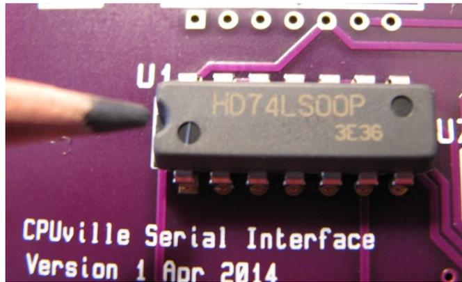
The ICs can be soldered directly to the board without fear of damage if you use a 15-watt or smaller soldering iron.
