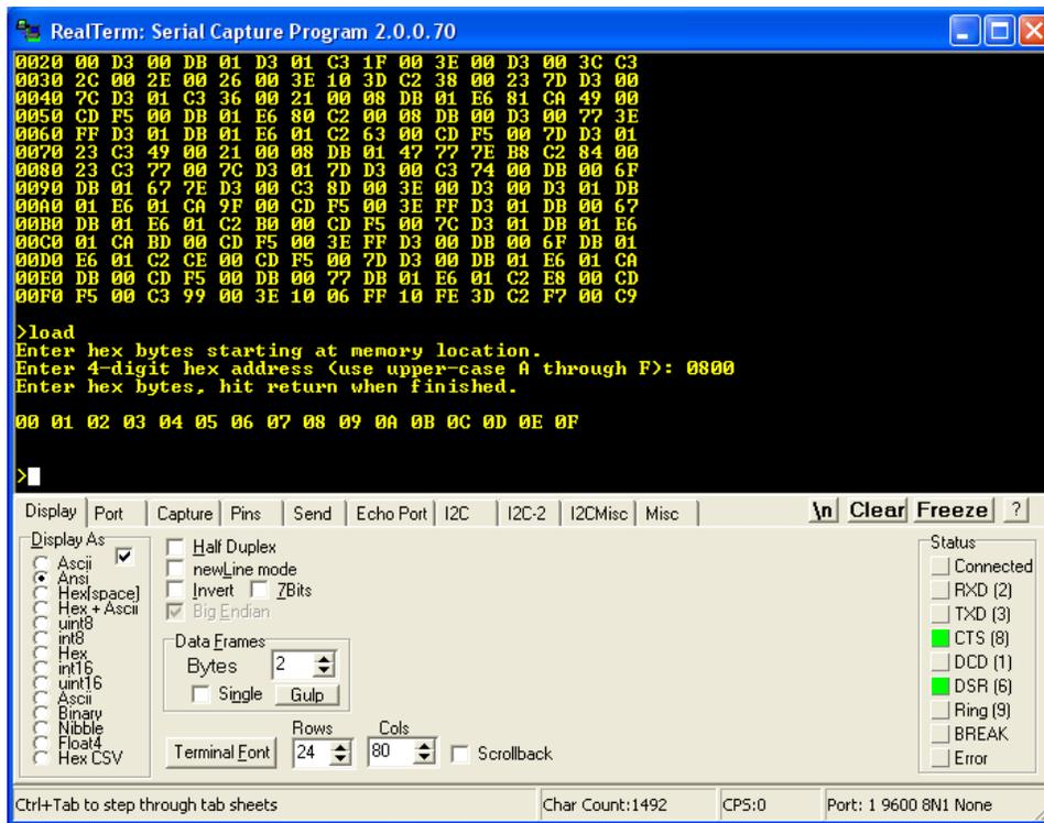
Here is a dump display of RAM starting at location 0x0800. You can see the 16 bytes I entered:
