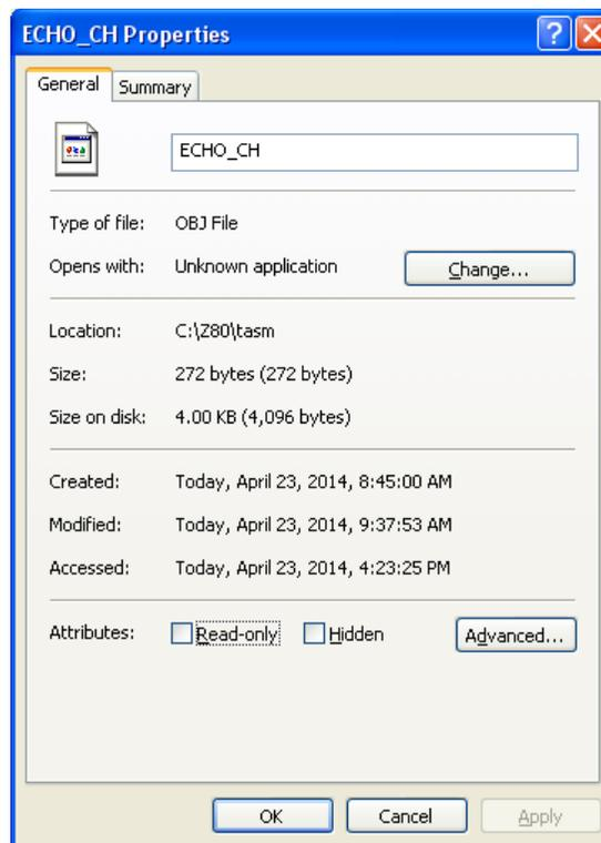
We see the file is 272 bytes long. Now we run the bload command, and enter the target address 0900h (no need to type the "h" in the monitor), and the length as decimal 272. Hit return after entering the length, and it lets you know it is ready to receive the file. Now, in the RealTerm Send tab, navigate to
