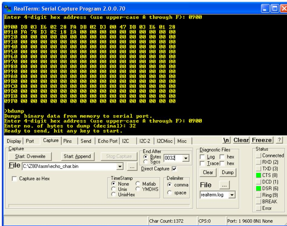
Click on the Overwrite button. The bottom of the display turns red, indicating that capture is underway. But, the Z80 computer has not sent any bytes yet.
